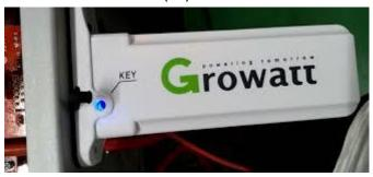
If the inverter is being installed inside a building, then you can entirely remove the small black rubber cover where it is marked 'Key'. If being installed where it might get wet, then leave the cover in place but peel it back as you will need to see the LED lights (Red, Green and Blue) during setup.
