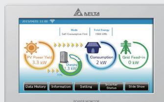
The Delta Smart Monitor features an interactive colour touch screen display, which allows the user to control the inverter and battery functionality. The Smart Monitor can be used to select one of the pre-programmed operating modes or to adjust the different time settings for purchasing and exporting energy to the grid. It also serves as a gateway for visualisation of data on mobile devices, such as the battery status, production, consumption, and exported energy.
